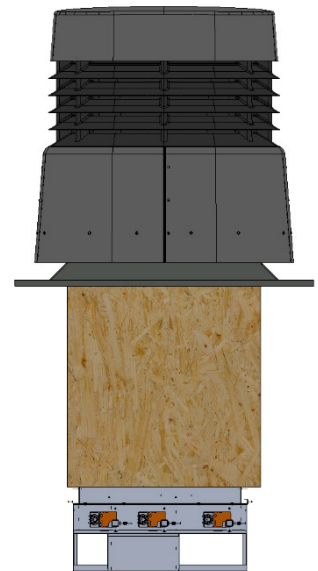
Figure 2 – Flat Roof Application with extended height
