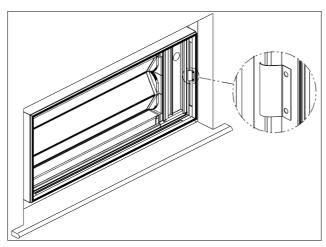
Should it be necessary to remove the louvre assembly for maintenance etc, depress the clips on either side whilst pulling the assembly out.
