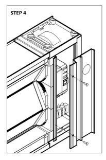
**STEP 4.** Remove the actuator cover from the front of the internal louvre module by removing the screws. Feed the cable through the grommet at the front of the internal louvre module, pulling the cable through the front of the actuator housing.
