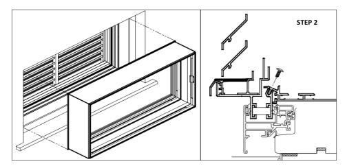
**STEP 2.** Insert the internal frame assembly to the external weather louvre and screw into place.
