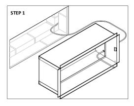
**STEP 1.** From the inside of the building, feed the power supply through one of the rubber grommets at either end of the wall sleeve. Enough cable should be left to allow connection to the junction box inside the actuator housing on the louvre unit. Insert the wall sleeve into the wall ensuring that the unit is the correct way up. Dependent on the size of the structural opening, it may be necessary to pack the sleeve to ensure it is positioned centrally within the structural opening.
