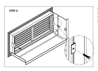
**STEP 3.** When the structural openings have been correctly aligned, secure the external louvre assembly to the wall sleeve with the fixings retained from earlier. Ensure that the fixings are fully tightened. The unit will now be fixed into the wall.
