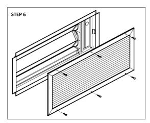
**STEP 6.** Insert the internal cover grille onto the aluminum sleeve. Once in place, secure with fixing screws provided.
